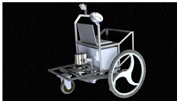
Figure 3-1 : CAD Rendering of Pushpak-2
