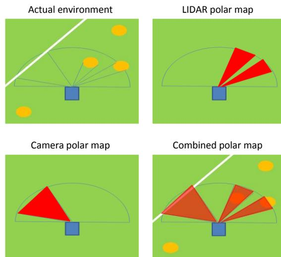
Figure 4-4 : Environment Mapping
