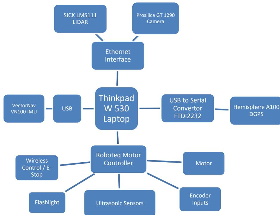
Figure 3-4 : Electrical Hardware Network
