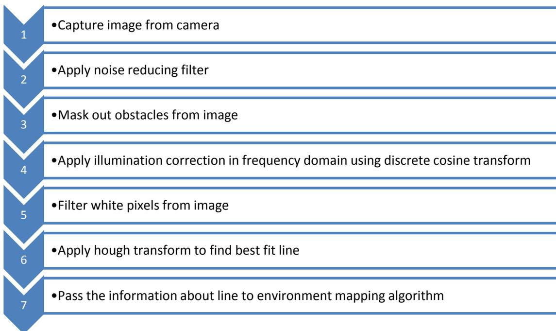
Figure 4-1 : Image Processing Algorithm
